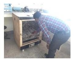
Sample Drying for Dry weight estimation
