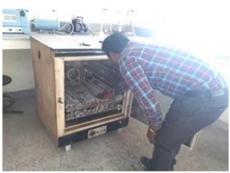
Sample drying for dry weight estimation
